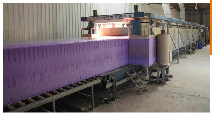
The FM300 is a high capacity machine for production of a continuous slab of flat top flexible PU foam with easy operation. Blocks of desired length can be cut with the help of a block cut-off machine at the end of the conveyor.
